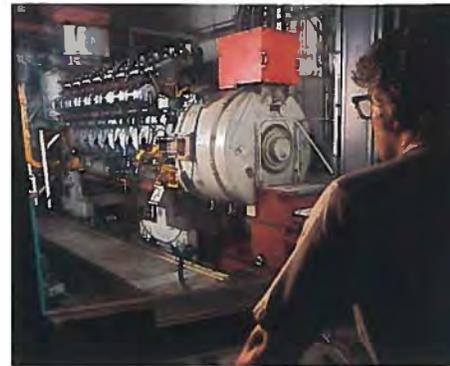
Computer-driven facility automatically cycles engine through complete test sequence.
