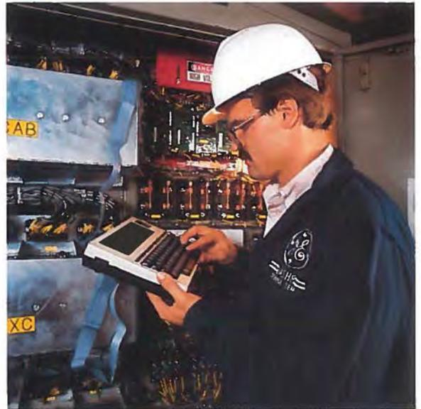
Operational data is transferred from locomotive computer memory to serve engineer's records.
