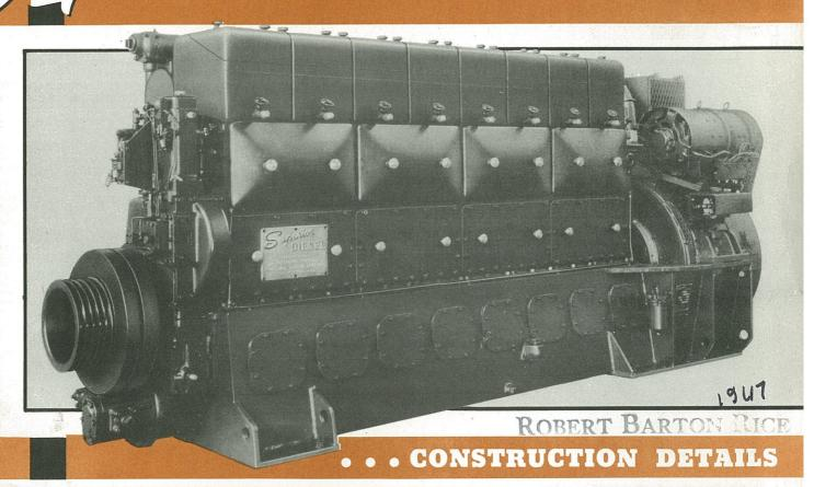
BEDPLATE is a steel welded design. It is provided with ribbed and flanged transverse members which are line bored with bearing caps to support the crankshaft in close alignment. The bedplate is extended to carry the generator as a single, rigid installation.
