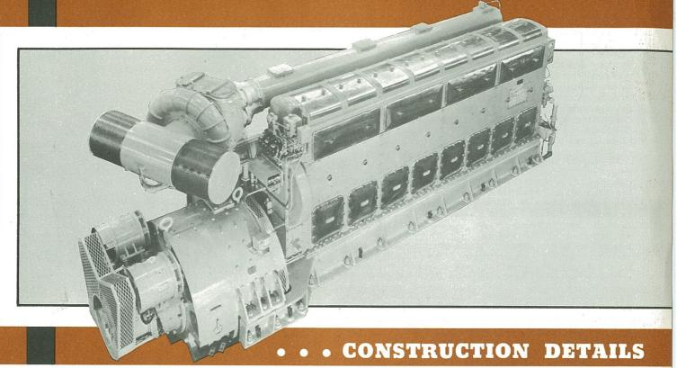
BEDPLATE is a steel welded design. It is provided with heavily ribbed and flanged transverse members which are line bored with their respective bearing caps to support the crankshaft is near perfect alignment. The bedplate is extended to carry the generator as a single, complete and rigid installation.
